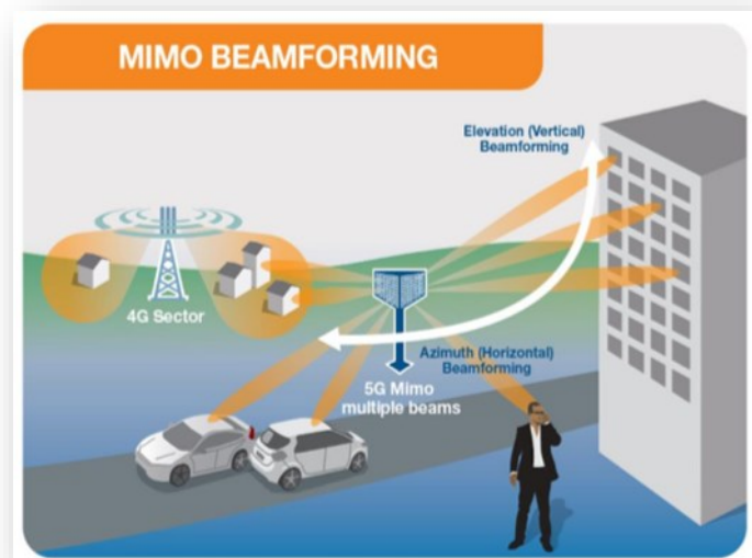
Fig: Massive MIMO beamforming and beam steering in a 5G network. [ITU-T Recommendation Series K Supplement 16 'Electromagnetic field compliance assessments for 5G wireless networks.]
